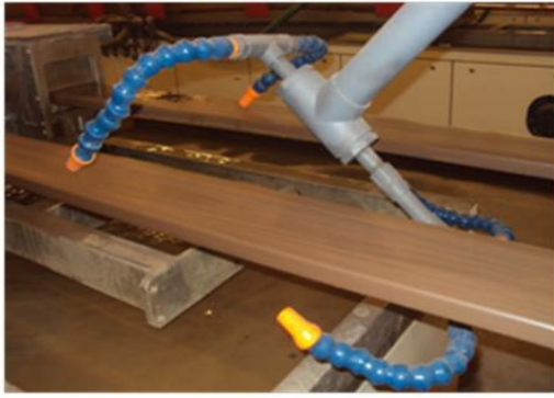
Low pressure nozzles blow moisture off boards from above and below.
