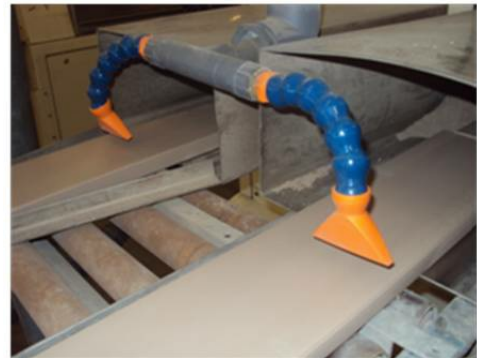
Particulate is blown from the product with fan shaped low pressure nozzles.
